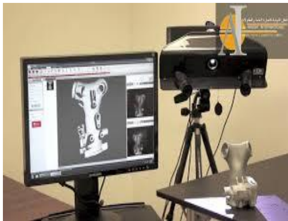
Picture (18) shows the relationship of the scanner with the product and the computer
