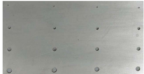
Fig. 6. photograph of holes machining at V=5 , I=15 time, 60 min, electrolyte 1M, gap distance 20mm
