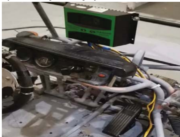
Fig. 3. Battery arrangement with MPPT controller
