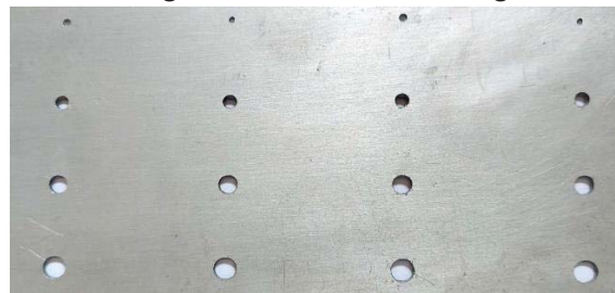
Fig. 4. Array holes 4,3,2,1 mm after machining at current 20Amp, 5 volt
