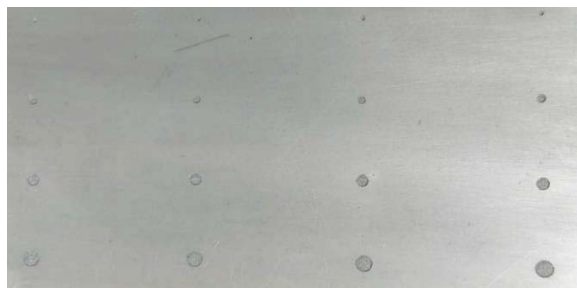
Fig. 8. photograph of array holes 1,2,3,4mm machining at V=5 , I=10 time, 60 min, electrolyte 1M, gap distance 20mm
