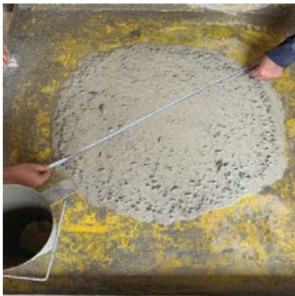
Fig. 7. Samples of T50 and slump flow tests
