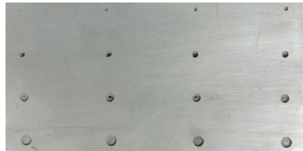
Fig. 7. Array holes 4,3,2,1 mm after machining at current 15Amp, 5 volt
