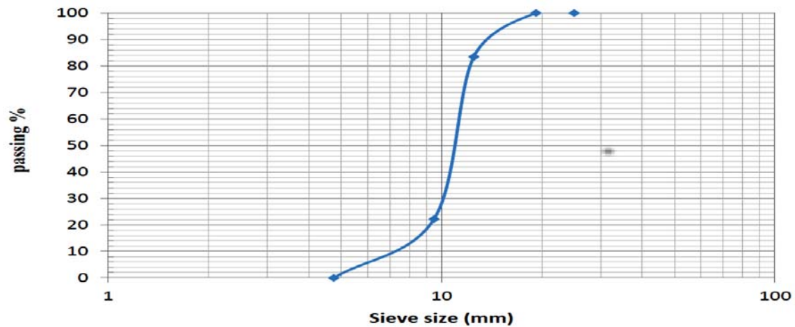
Fig. 6. Grading of crushed coarse aggregate
