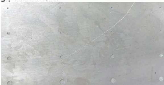
Fig. 9. photograph of array holes 1,2,3,4mm machining at V=5 , I=5 time, 60 min, electrolyte 1M, Gap distance 20mm
