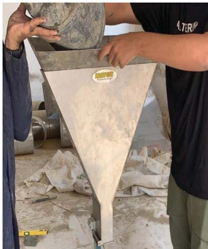
Fig. 9. Sample of V-Funnel test
